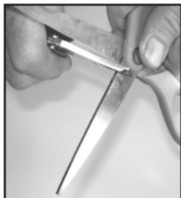
In the case of removing burrs from scissors or shears, do not do anything to the flat side of the blade with the sharpener. Simply use finger pressure to spread the blades as you close the tool, then reverse the pressure (i.e. forcing the blades to rub each other) to open the tool. This will remove the burr without damaging the cutting edge. You do not ever want to put any bevel on the unbevelled side of the scissor blade as it will harm the cutting action.
